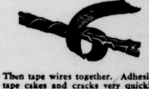
Then tape wires together. Adhesive tape cakes and cracks very quickly.
