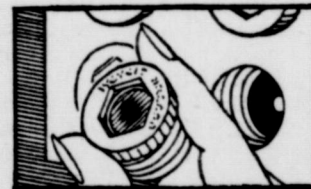
Unscrew the "blown out" fuse, touching only its top. You can tell it by the burned patch in the window on top of fuse.
