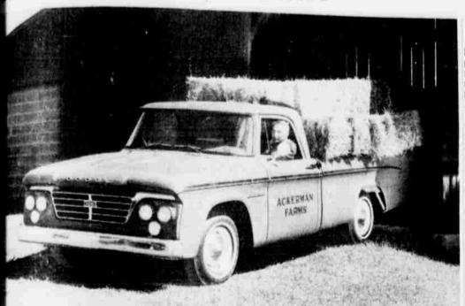
TRUCK STYLE LEADER-At home in the city and on the farm, the 1962 e D-100 Sweptline pick-up features a handsome one-piece stainless steel grille, hood silhouette and contemporary styling. A highlight of the Sweptline is its horsepower, 225-cubic-inch, Inclined 6-cylinder engine. The unit is available a 114-inch wheelbase and 612-foot body or a 122-inch wheelbase and 8-foot
