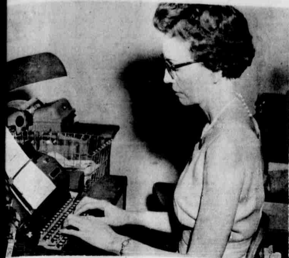
TELETYPESETTER --Above is the teletypesetter which converted news onto rolls of tape, which in turn were mounted on the Intertypemachines to produce column width galley copy. The tape activated the Intertypemachine. Shown operating the tape machine above is Mrs. Treva Quigley.
