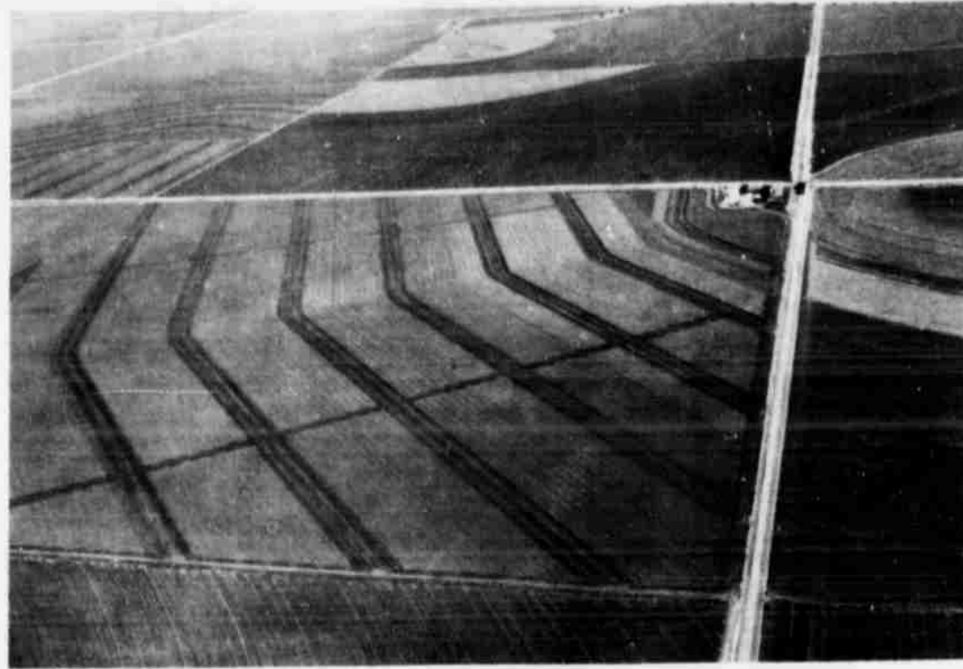
PARALLEL TERRACES such as these were the biggest advancement made the past two years by the Lamb County Soil Conservation District. During 1966, 144,565 feet of parallel terraces were constructed in the district.
