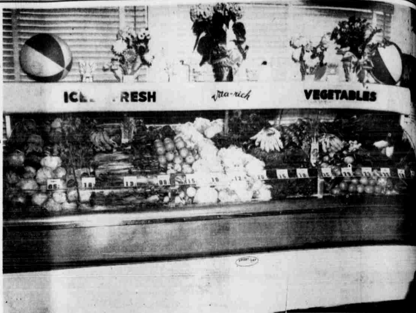
A FRONT VIEW OF THE VEGET ICER in use at Houk Bros and displaying a lovely selection in fresh vegetables. Note the dark section just below the vegetables, about six inches deep, and you can visualize the ice vault extending all underneath the vegetables, cooling them Nature's Way.
