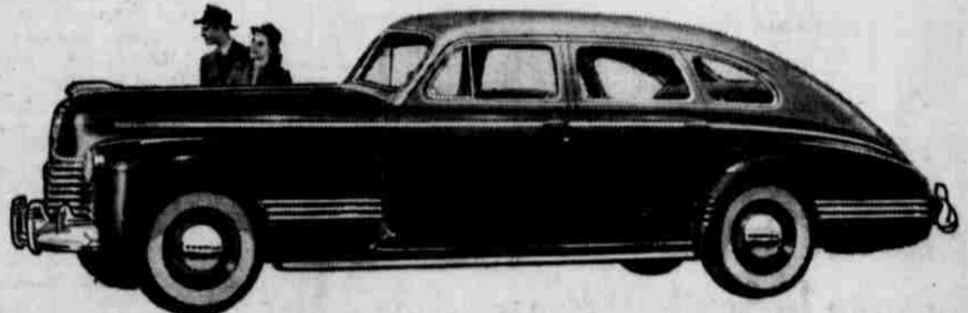
PONTIAC STREAMLINER "TORPEDO." A new streamlined version of Pontiac's famous "Torpedo" styling. 122-inch wheelbase—7 1/2 inches greater over-all length. New concealed running boards. Offered in the Four-Door Sedan and Sedan Coupe.
