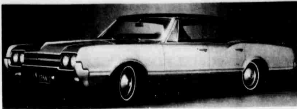
Oldsmobile's introduction of the Cutlass Supreme for 1966 brings a four-door hardtop to the F-85 line for the first time. Displaying the same "Hollywood" styling of the full-size, four-door Oldsmobile, the Cutlass Supreme features an extra-luxurious interior and optional vinyl-clad roof. Like all of the Cutlass models, the Supreme is powered by the 10.25-to-1, 330-cubic-inch Jetfire Rocket V-8 which may be teamed with the highly efficient Jetaway automatic transmission.
