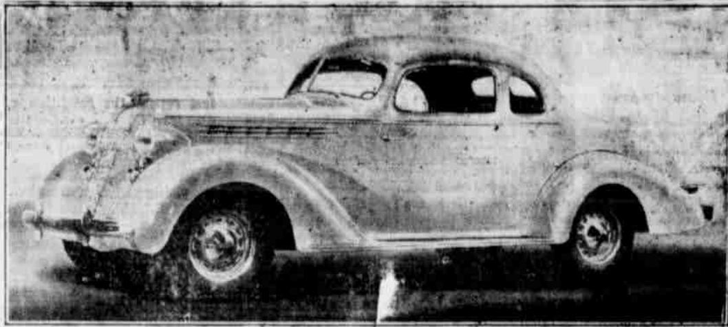
The 1936 Terraplane Coupe mounted on 115-inch wheelbase, with an 88-horsepower engine standard, with 100 horsepower optional with the high compression aluminum cylinder head.
