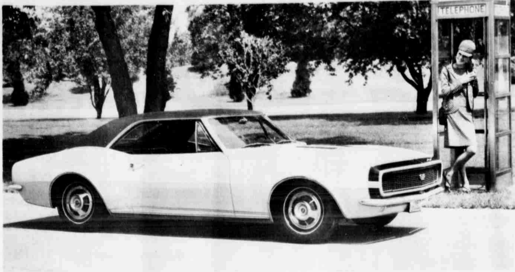
1967 CAMARO SUPER SPORT COUPE -- The all new CAMARO will be built in sport coupe and convertible models. The Camaro line incorporates many sprightly options that include concealed headlights behind a lattice grille which opens and closes when lights are turned on and off, plus a hood with simulated louvers and a wide "bumble bee" paint band on the nose. A 350-cubic inch V-8 engine is used in the Super Sport version of the CAMARO. They go on display today at Armes Chevrolet.
