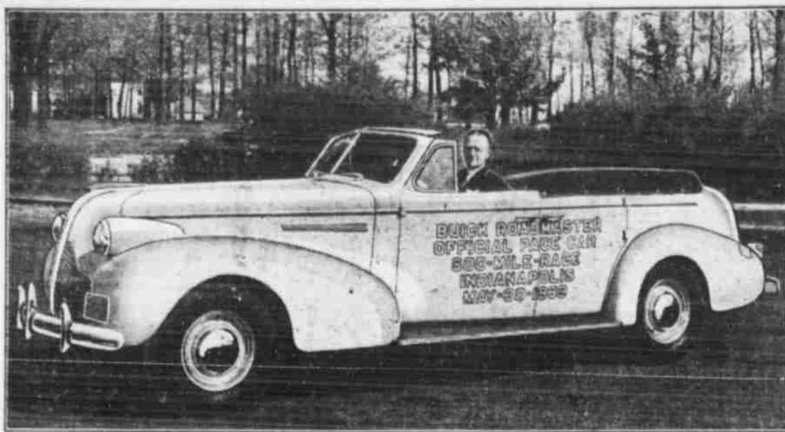
BUICK HAS been chosen this year to pace the fast field in the 27th annual Indianapolis Motor Speedway race May 30th, and the car picked by Buick Chief Engineer Charles A. Chayne (seated at wheel) is this Roadmaster convertible phaeton, powered by a 143-horsepower valve-in-head straight 8 engine. The car is a stock Buick model and is capable of speeds upward of 100 miles an hour. Mr. Chayne will drive with T. E. (Pop) Myers, vice president and general manager of the Speedway, as a passenger.
