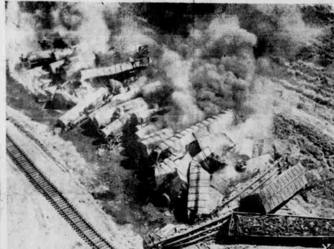
SMOKING WRECKAGE—Thirty-five cars, some of them containing oil and gasoline, piled up high and sideways near Corsicana, Tex., before bursting into flames. The cars were part of a 62-car Fort Worth and Denver freight that was derailed. Damage was estimated at over $300,000, but no one was hurt. At lower left is a section of new track hurriedly built around the wreckage to let other trains pass. —AP Wirephoto
