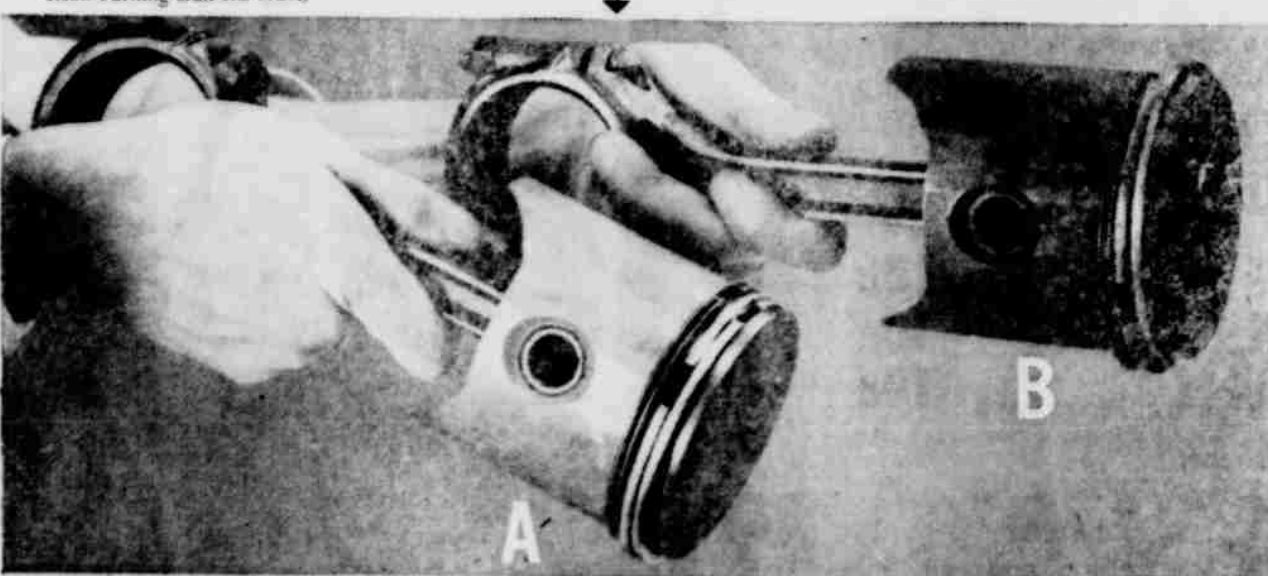
Compare clean piston "A" from engine using new NO-NOX with piston "B" from engine using the "dirty-burning tail-end" of gasoline that Gulf refines out. Both pistons shown here, from Gulf test engines, ran the same number of hours under the same conditions.
