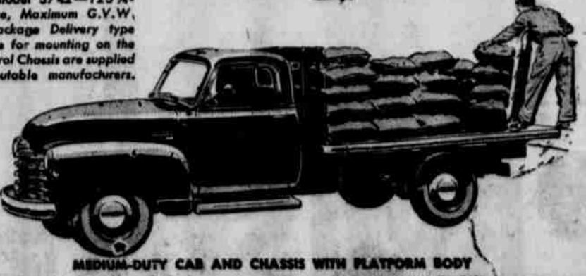
MEDIUM-DUTY CAB AND CHASSIS WITH PLATFORM BODY Model 3808—137-inch wheelbase, Maximum G.V.W. 8,900 lb.
