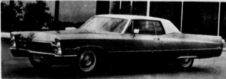
EXTERIOR CHANGES in the 1968 Cadillac, as shown in this Coupe de Ville, include a new grille and larger parking lights in the front, redesigned cornering lights and new marker lights on the side plus a new deck lid and all chrome bumper in the rear. On the inside, safety related product improve-
