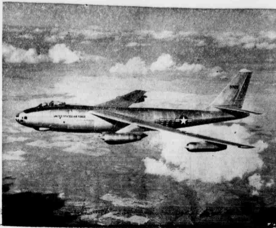
The B-47, a U.S. Air Force jet bomber that can fly 3,000 miles, sold its bomb load and return, is shown in flight. It can fly at 600 miles per hour, plus. Only three men are in the crew: a pilot, co-pilot and a navigator-bombardier-observer. They do the job of 10 men in a B-29 or 15 men in a ten-engine B-36. The B-47 has six jet engines. A load of 20,000 pounds of bombs can be tucked into the B-47's bomb bay. U.S. Air Force Photo from Associated Press.
