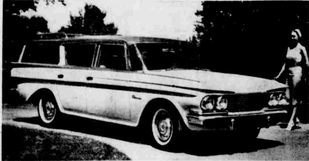
A HANDSOMELY RESTYLED GRILLE and new hood lines distinguish the 1961 Rambler Classic station wagon, available in three-seat and two-seat models. Fresh sculptured side styling accents the compact Rambler's new front-end design. Engines in the Classic series include the lightweight aluminum six-cylinder engine rated at 127-horsepower and the V-8 engine developing 200 horsepower.
