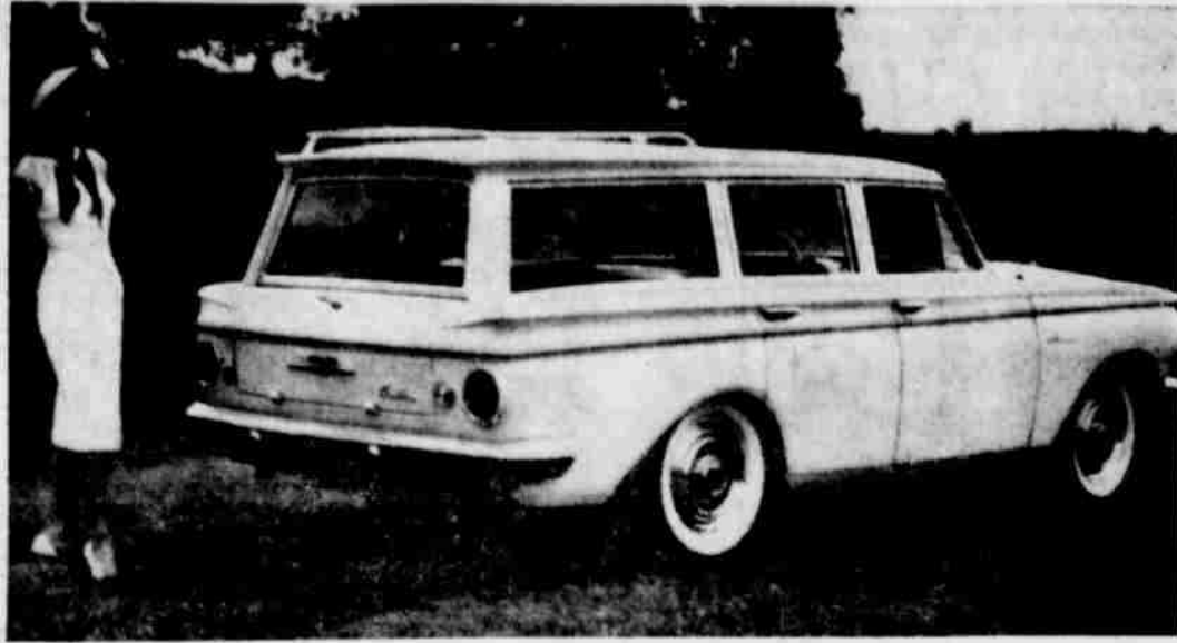
THE RAMBLER AMERICAN four-door station wagon, a new model for 1961, features the roof-top luggage rack, a trademark of Ramblers for several years. The rear luggage opening is two inches wider than on past models. The upper section of the tailgate, which can be set in three positions, is framed in extruded aluminum. All models have substantially greater glass area in 1961. Station wagon cargo space is increased 23 per cent to 64 cubic feet.
