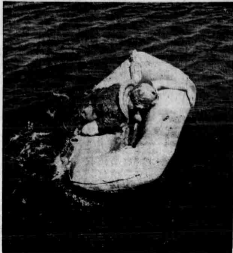
One-man rubber life rafts are standard equipment in all Navy single-seat fighters. The raft is packed and stowed below the turtle back immediately behind the pilot's seat. After a landing at sea, the pilot pulls out the raft, turns the valve on the bottle of carbon dioxide, and the raft inflates in 1 minute. To get onto the raft, the pilot grabs the opposite side and throws himself horizontally across the boat.
