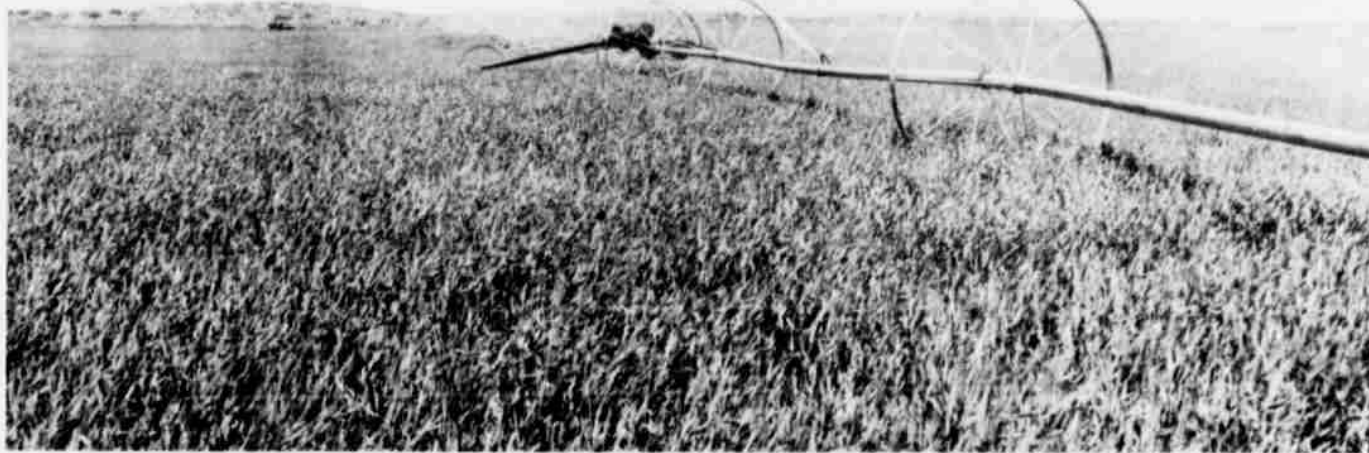
LARGE SPRINKLER OPERATION -- Above is a wheel type, self propelled sprinkler system used on the Cleo (Sonny) Whitmire farm located 4 1/2 miles north of Sudan. This is a quarter mile, five-inch lateral being used to apply water to a Barley crop which will be used as winter pasture and then harvested for grain.
