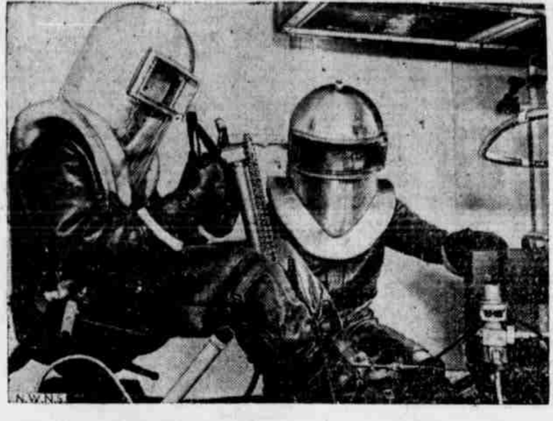
Garbed in fantastic aluminum helmets and heavy fleece-lined horse leather suits, "cold room" workers test hydraulic control system of a high altitude bomber in the Douglas Aircraft plant at Santa Monica, Calif. Here a scientific ice box has been built that can create a temperature of 104 degrees below zero.
