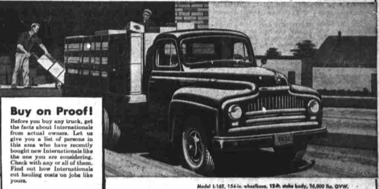
Model L-162, 154-in. wheelbase, 12-ft. stake body, 16,000 lb. GVW.
