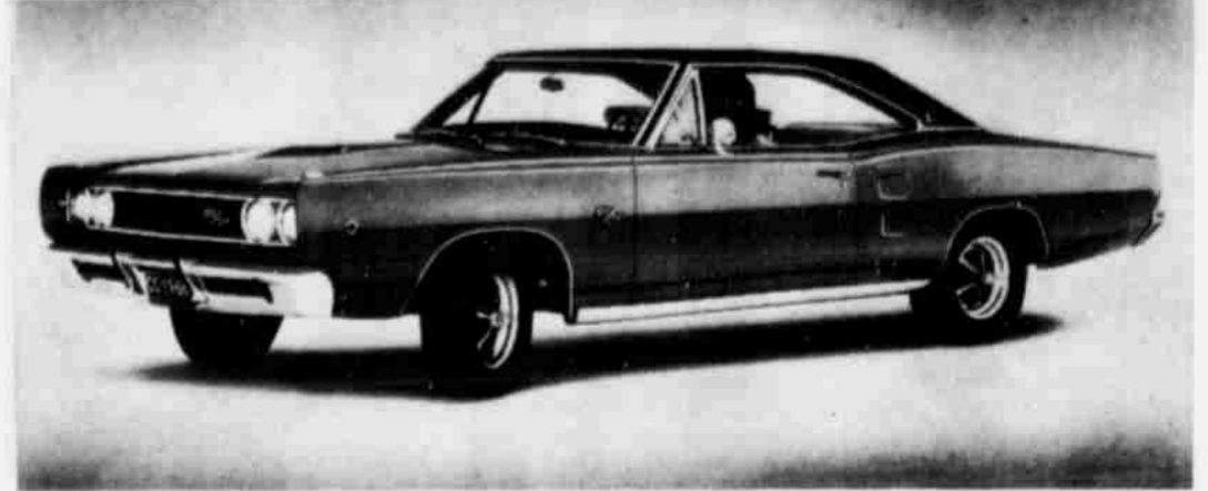
1968 CORONET will bow at Garland Motor Co. today. The family-size series has a 117 inch wheelbase -- big enough for comfort, small enough to park. Above the Coronet R/T which features rally suspension and a 440 cu. in. engine as standard is available in hardtop and convertible models.
