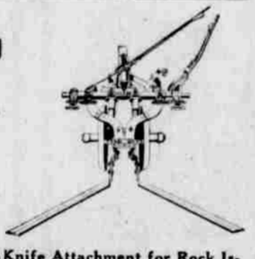
Knife Attachment for Rock Island No. 126 Lister Cultivator.
