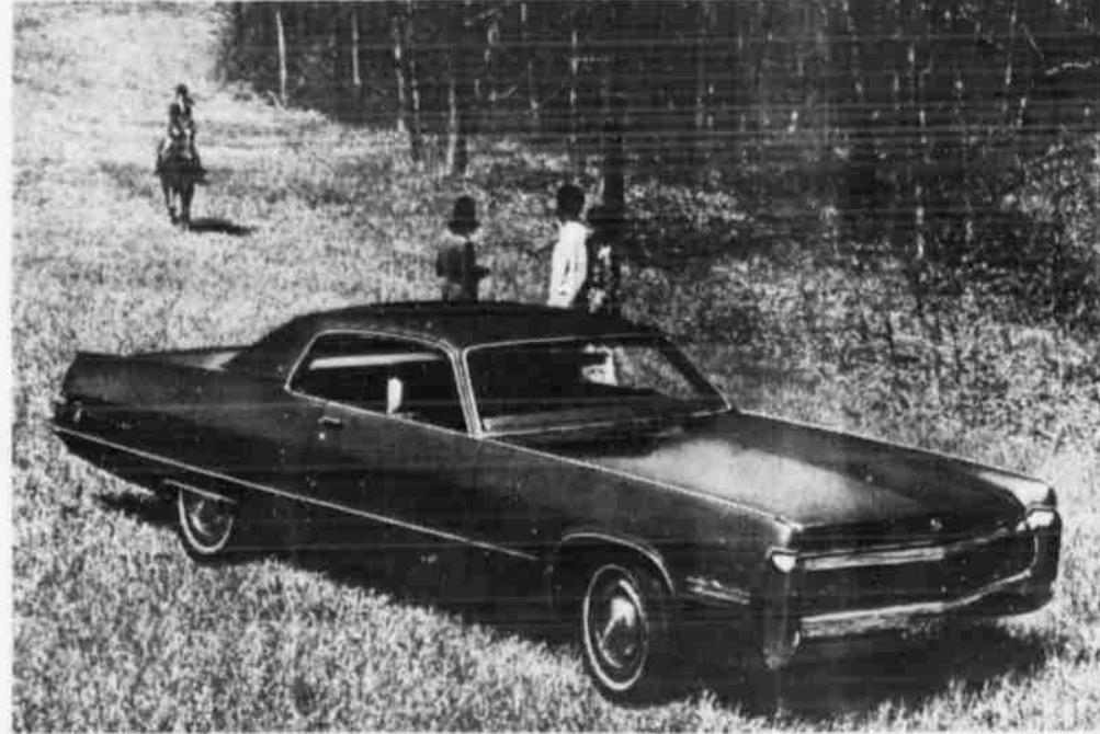
LONG, LOW AND LUXURIOUS —The Chrysler Imperial LeBaron enters 1972 as an all-new luxury car with simplified but elegant lines. In two and four-door hardtops. Wheelbase: 127 inches. The standard engine is a 440-cubic-inch V-8.
