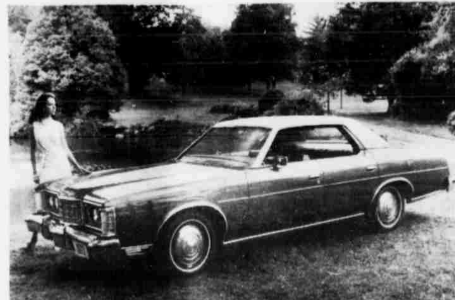
Most changed Ford Division car for 1973 is the full-sized Ford. Shown here is the LTD four-door hardtop. All-new sheet metal below the window line and a new segmented grille give the 1973 Ford a more formal look. All 1973 Fords have a new impact-absorbing bumper system, although the overall length of the car is increased only about one inch. Power front disc brakes, power steering, SelectShift Cruise-O-Matic transmission and a 351-2V eight-cylinder engine are standard in all new Fords.
