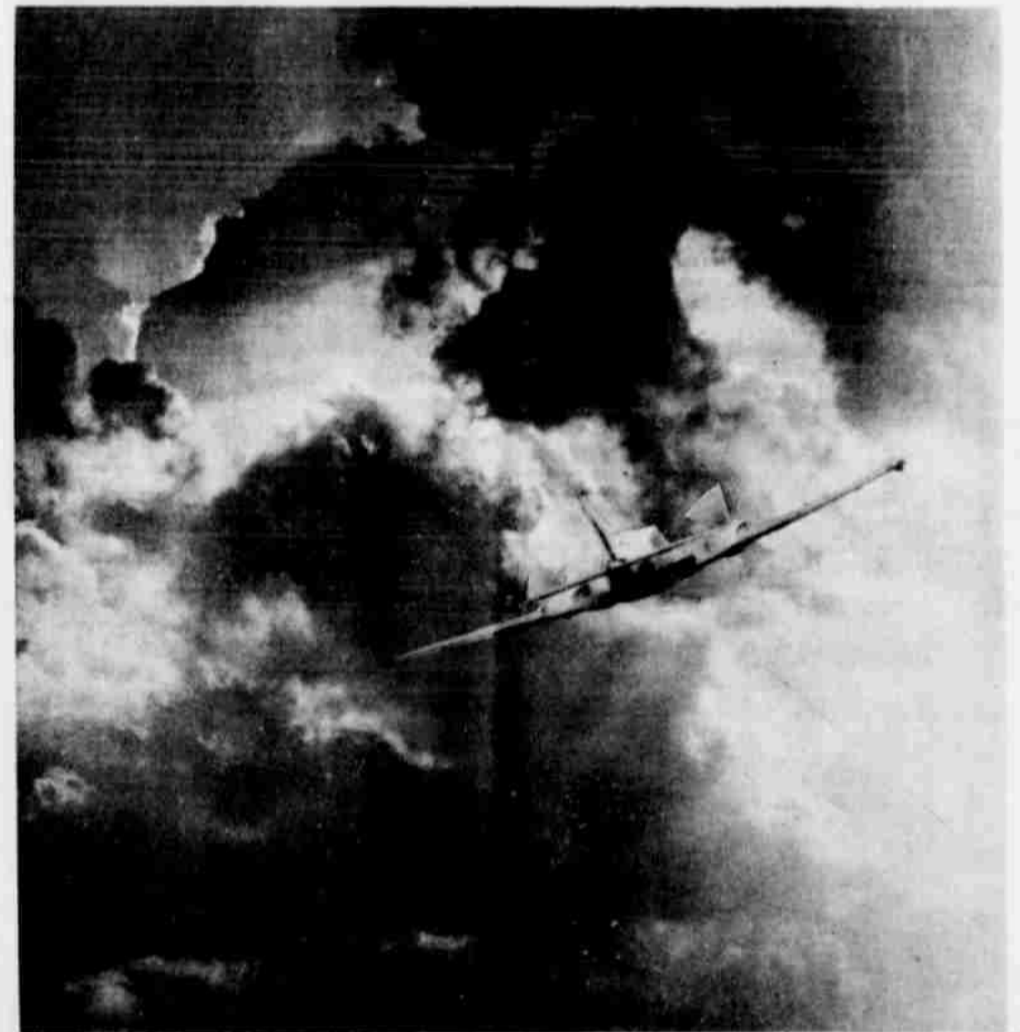
SINCE HAIL SUPPRESSION operations began May 14, personnel have averaged working more than 10 storm cells per day. Silver iodide is fired into hail-filled clouds through wing-mounted pyrotechnics controlled by the pilots. This is one of the three twin-engine planes used in the program. (Photo by Plainview Daily Herald)
