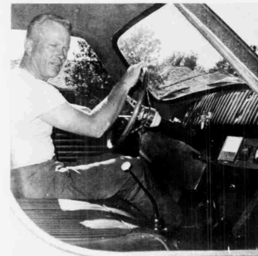
INTERIOR design, all hand-built, of the EMV ElectriCar prototype is shown by Cotton Whatley. The final design will meet all federal safety regulations, he says, and be as comfortable as "anybody would want." Note the gear shift in the floor. It has three speeds forward and a reverse, unique for any electric car ever built.
