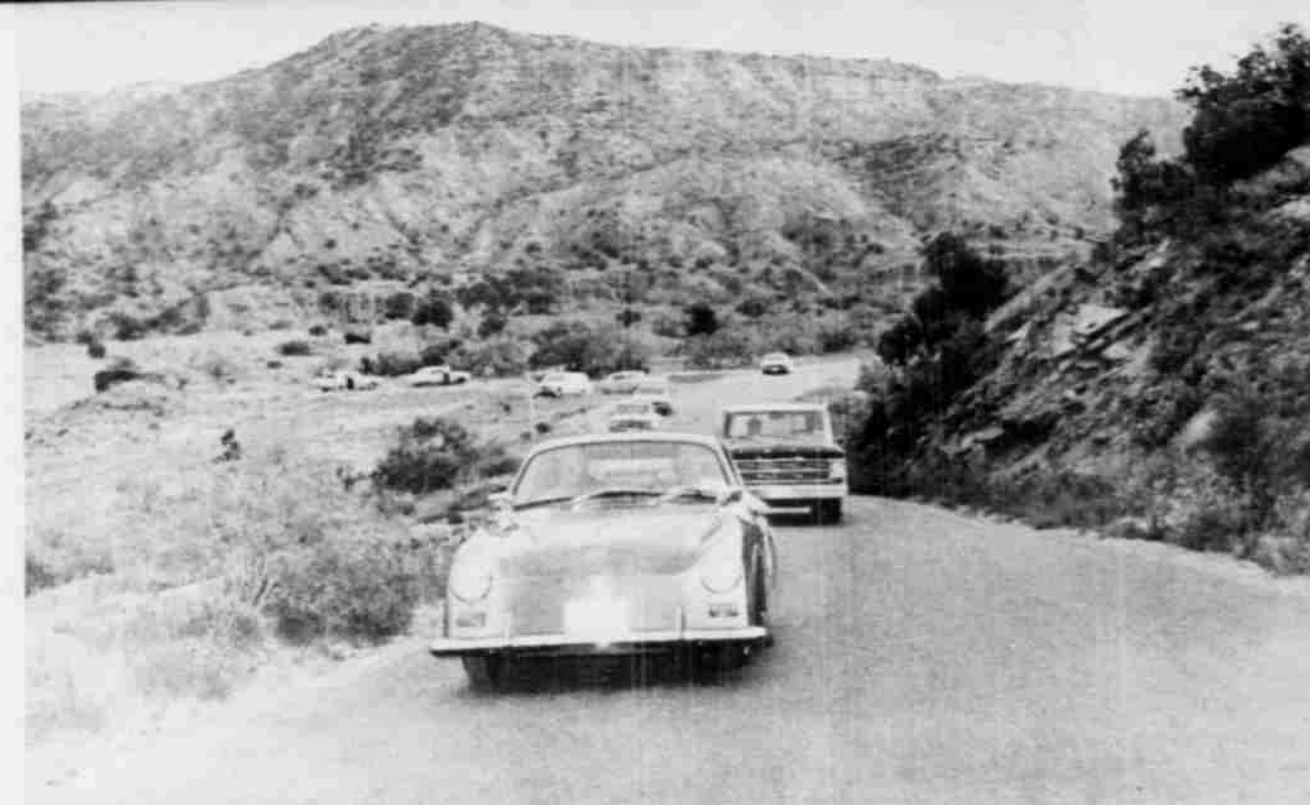
STARTING UP Palo Duro Canyon, the 2000-pound car, driven by a 5-horsepower electric motor, began a 700-foot ascent in 1.1 mile. EMV's ElectricCar made the grade with ease.
