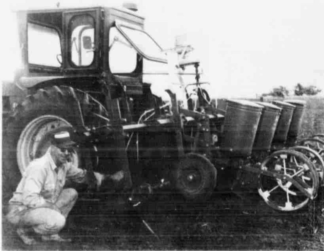
THREE-WAY RIG. Bill Elms of Amherst in Lamb County accomplished three separate operations in a single pass over his cotton land this spring with the planting rig shown here. In addition to shaping beds and bed planting, Elms attached deep-running chisels to a second tool bar to deposit a fumigant to control nematodes. Chisels (like the one in front of his hand) were set to deposit chemical about 4" deeper than opening plow. Elms fumigated 100 acres this year after soil tests indicated he had a nematode problem. He had tests made after his yield dropped from a high of 1242 lbs. of lint per acre in 1962 down to where "it's all I can do to make a bale and a quarter."
