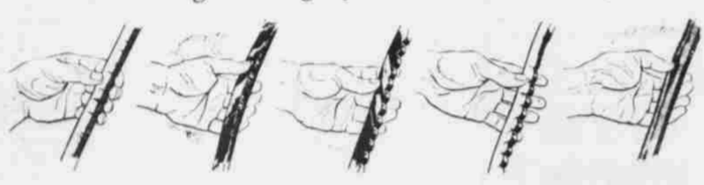
Crack on underside, enlarged by flexing belt. Can break any time. Grease softened inner core, slick sides cause slips, rot rubber. Belt with stick, hard sides slips, causes low battery, overheating. Peeling inner core top; sides and bottom surfaces, will soon fail. Belt looks okay from top; sides and bottom may be split, worn.
