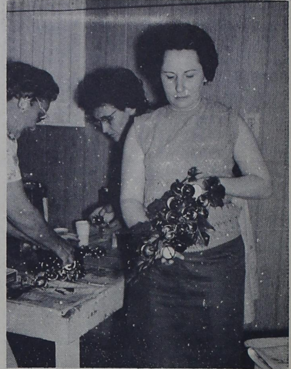
FINISHED PRODUCT -- Dorothy Dudley displays a grape cluster which has just been completed, while Eula Mae Madole assists Mildred Hill in breaking the grapes from the mold in which the resin is poured to set.
