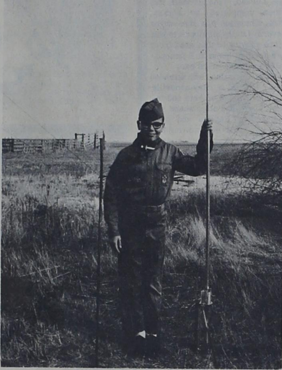
"THIS IS ALL IT TAKES" -- For an antenna, operator Gregory uses a coil-loaded vertical, only sixteen feet in height. Although this antenna cost Randy less than $20, it has the capability to send and receive a signal from around the world.
