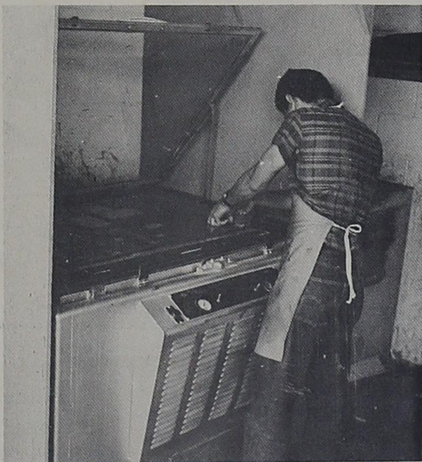
Page negatives are printed on thin photosensitive aluminum sheets by an tonization process. (PHOTO By Bob Burmeister)
