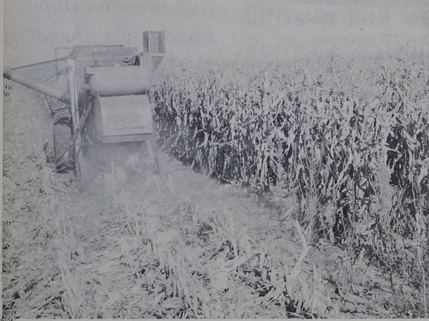
Beautiful weather made for ideal harvest conditions as the picker-sheller rumbled down through the field making a clean sweep of two rows at a time. The corn was dry--around 14% moisture.
