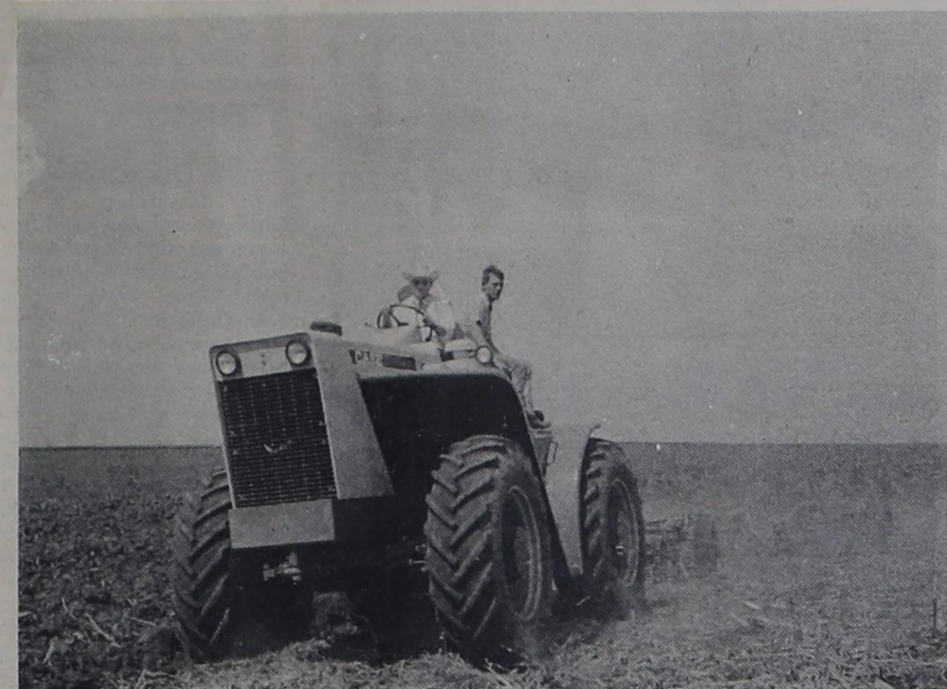
LUGGING EIGHT 16-INCH MOLDBOARD PLOWS, the Case 1200 demonstrated by Oklahoma Lane Farm Supply last week churns through the land for three visitors on board to see how it's done. The plows were set for an 11-inch draft.
