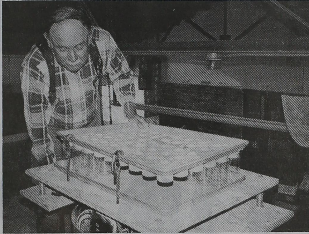
He can fill 54 containers at one time. Underneath, there's a motor which vibrates and helps mix up the contents.
