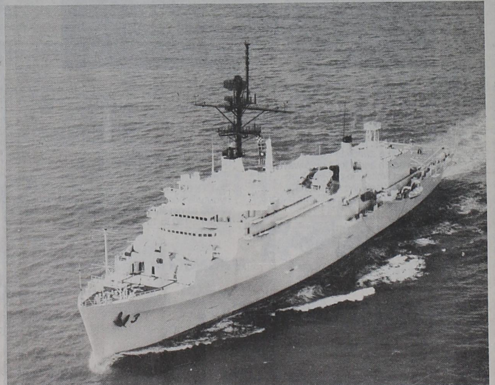
"The Great White Ghost of the Arabian Coast" USS LaSalle is the only ship in the U. S. Navy painted entirely white. This aids in keeping the ship cooler since she is permanently home based in the Middle East area.
