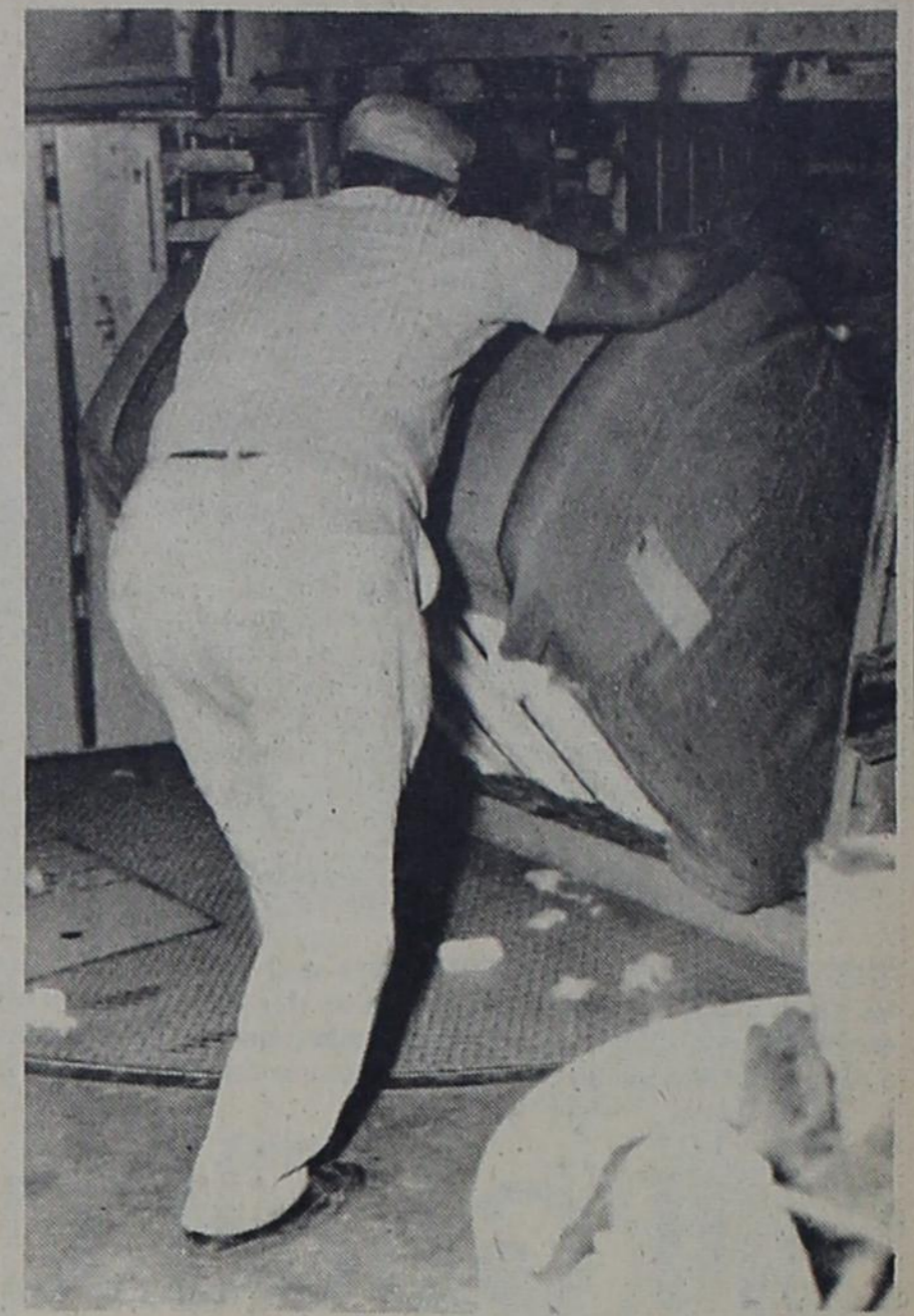
AND OUT SHE COMES--Tremendous pressure is exerted in this big double press which forms the finished bale. Here a workman tumbles out the bale that was seen entering the gin from the trailer outside. It takes about eight minutes to gin a bale.
