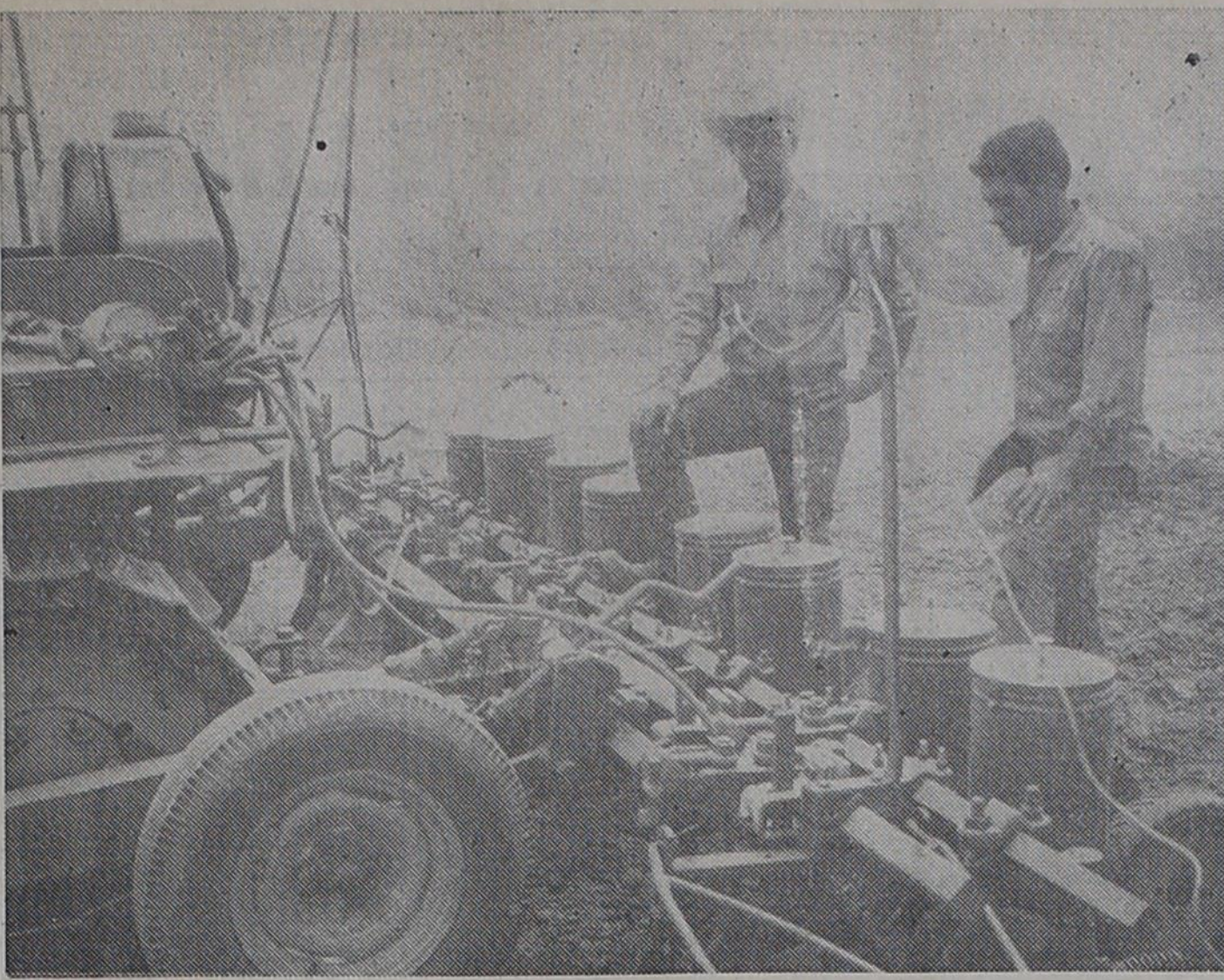
A three-in-one implement is being used on the James Readhimer farm in northeast Parmer County to apply anhydrous ammonia, plant and cultivate at the same time. Readhimer, with hat, and a farm hand stand behind the implement which is hooked to a D4 cat.
