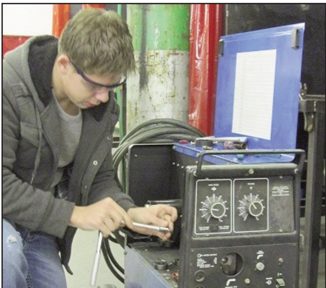
Aaron Massey studies proper shop equipment maintenance procedures as he services a MIG welder.
