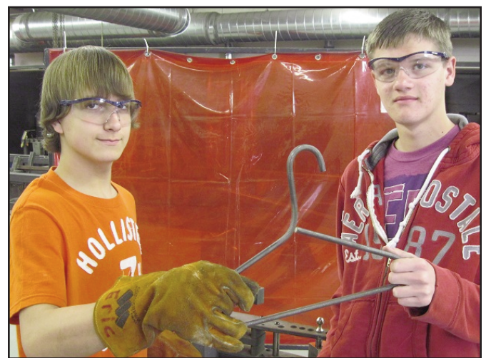
Braxton Dow and Justin Jenkins show the work that they and Kendall Naceanceno created. The hangars, made of 3/8" steel rod, will be used to store the vocational ag shop's leather welding jackets.
