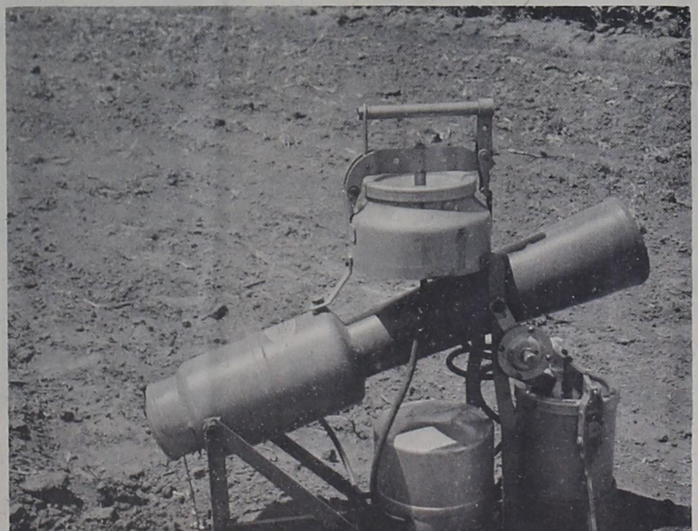
SHOO BIRDS -- This piece of equipment is the modern replacement for the scarecrow. The device utilizes carbide gas to emit a loud bang every ten minutes or so and does an effective job of keeping the birds away from the crop. This particular device was put into use by Nathan Tharp of Texico.
