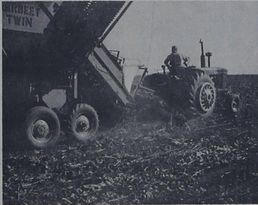
FULL SPEED AHEAD -- This sugar beet digger on the Marlon Inman farm, five miles southeast of Farwell, was operating "full speed ahead" on Friday morning. The digger pulls the beets from the ground and cuts away the tops in one operation.
