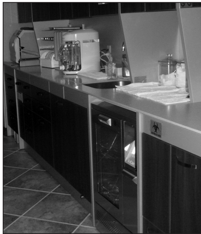
An autoclave to keep instruments clean, and water filters to clean up water before it gets used on patients.
