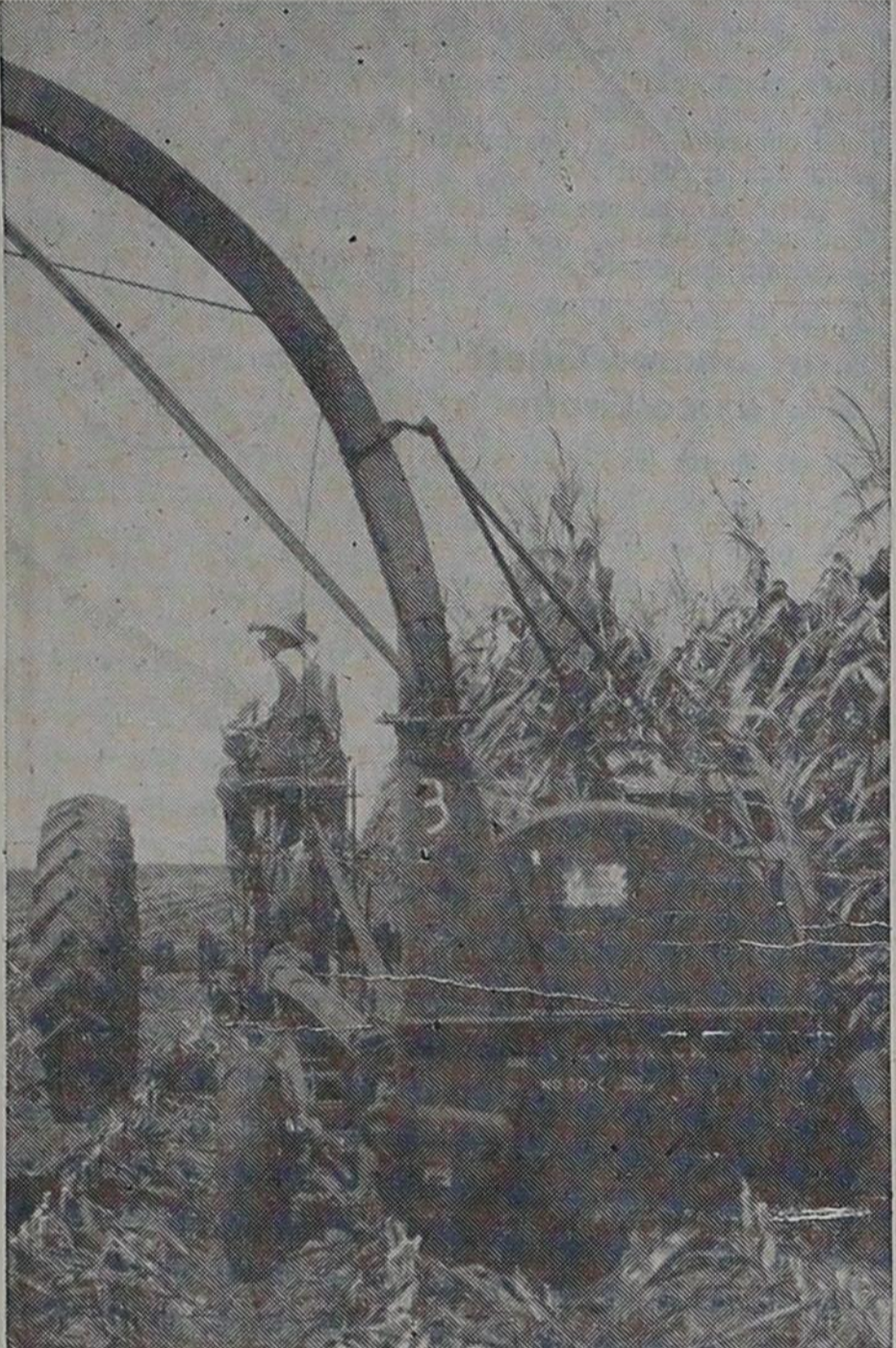
Cleaning up a field the quick way is how a whirling silage cutter works. Here tall corn is being cut from the farm of Mose Glascock, south of Farwell. Nothing is left except the short stumps of the corn stalk and the rest is whisked away to storage by a truck. Glascock's corn is making 18 tons per acre, the yield having been reduced by severe worm infestation.
