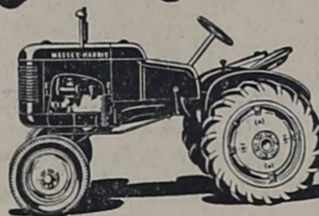
3-4-Plow 44—260-cubic-inch, 4-cylinder engine, 5 speeds forward.
