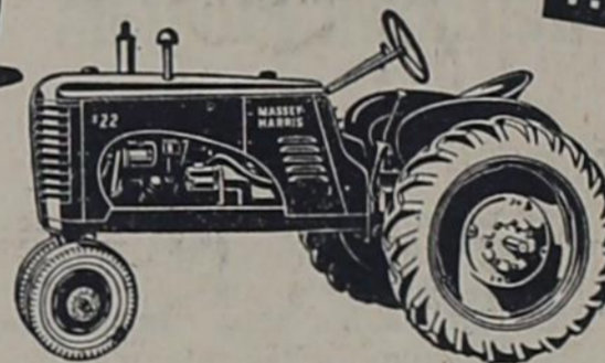
2-Plow 22—140-cubic-inch 4-cylinder engine, 4 speeds forward.
