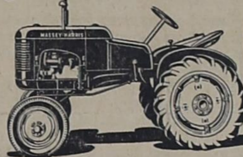
3-4-Plow 44—260-cubic-inch, 4-cylinder engine, 5 speeds forward.
