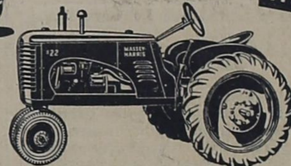
3-4-Plow 44—260-cubic-inch, 4-cylinder engine, 5 speeds forward.
