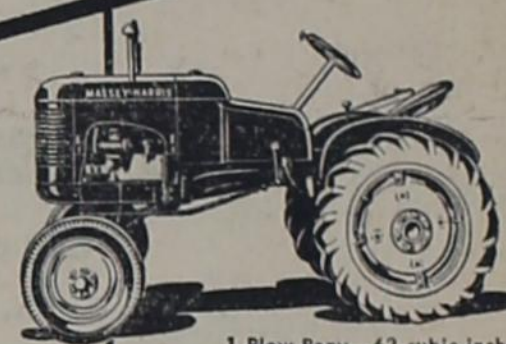
1-Plow Pony—62-cubic-inch, 4-cylinder engine, 3 speeds forward.
