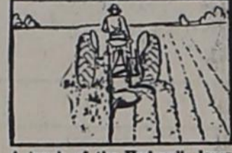
A touch of the Hydraulic lever lowers plow. Automatic control of depth made possible.
