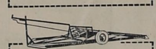
MODEL 12—Width 12', length 21', cutting blade length 9' 3", depth 16", 3 plow tractor. Model 9 shown at top of page slightly smaller for 2 plow tractor.
