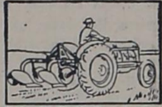
Hydraulic Touch Control raises plow for easy turning, and fast transport on road.
