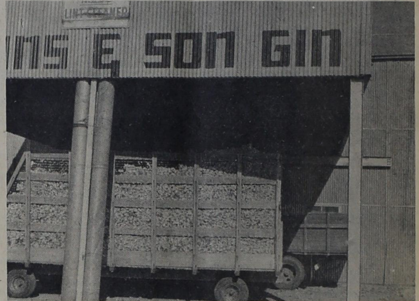
THIS IS THE BUSINESS END of one of the Lazbuddie area gins, which have been running around the clock to get the 1959 crop out. Folks not familiar with cotton production are constantly amazed by the giant suction pipes that pick up bolls for ginning.
