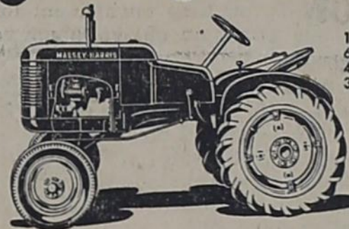
3-4-Plow 44—260-cubic-inch, 4-cylinder engine, 5 speeds forward.
