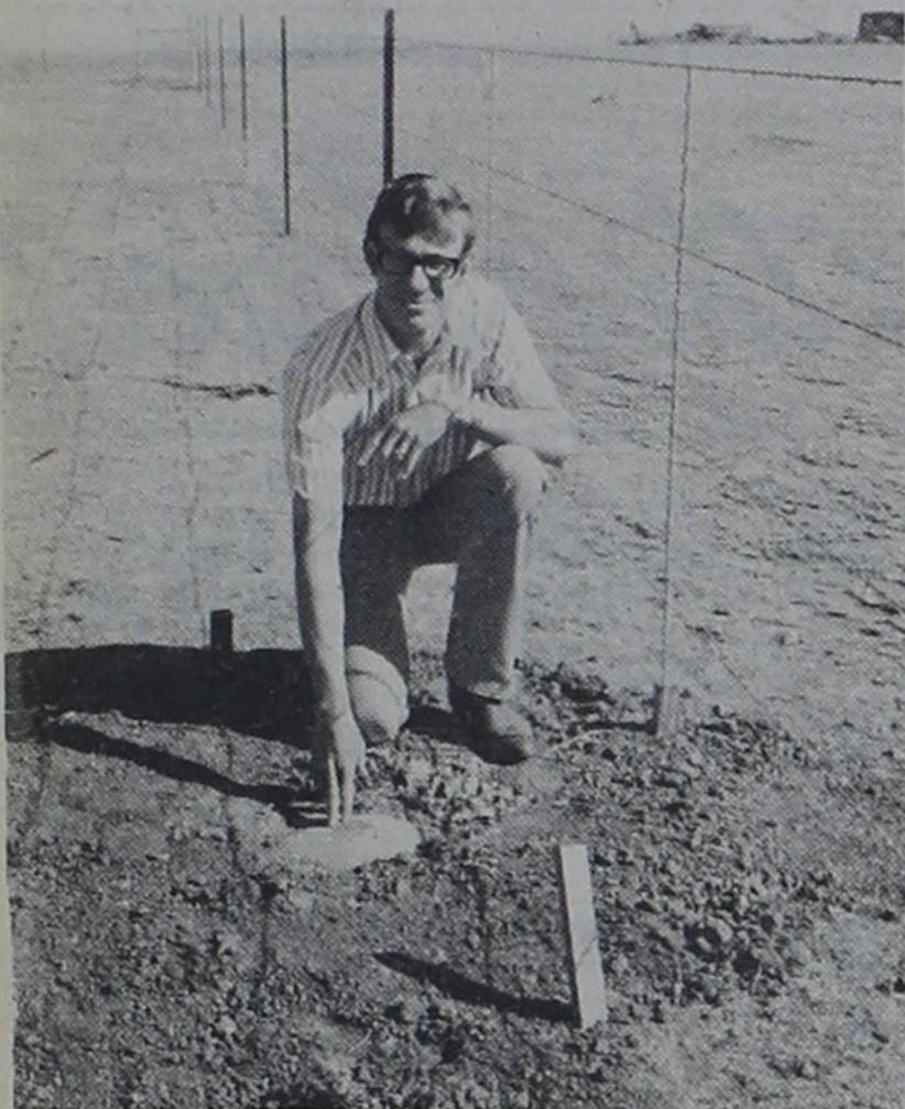
CHECKING A MARKER - Edwin Livingood of the Friona SCS office checks a permanent altitude marker set at the damsite near Bovina. At this particular location, the altitude is 4100.07 feet above sea level. The marker is one of three permanent markers at the dam.
